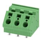
PCB terminal block, nominal current: 32 A, rated voltage (III/2): 630 V, nominal cross section: 4 mm², number of potentials: 3, number of rows: 1, number of positions per row: 3, product range: ZFKDS(A) 4, pitch: 10 mm, connection method: Spring-cage connection, mounting: Wave soldering, conductor/PCB connection direction: 45 °, color: green, Pin layout: Linear pinning, Solder pin [P]: 4.6 mm, number of solder pins per potential: 2, type of packaging: packed in cardboard
