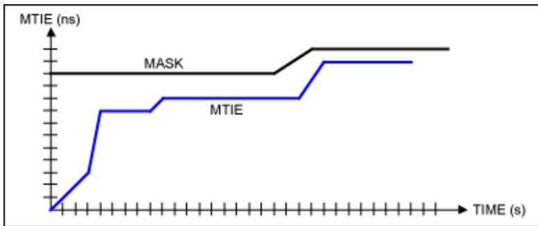
Figure 6. Typical MTIE graph with an MTIE mask.
