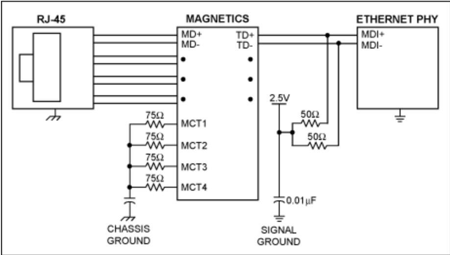
Figure 3. Typical Ethernet PHY connection.
