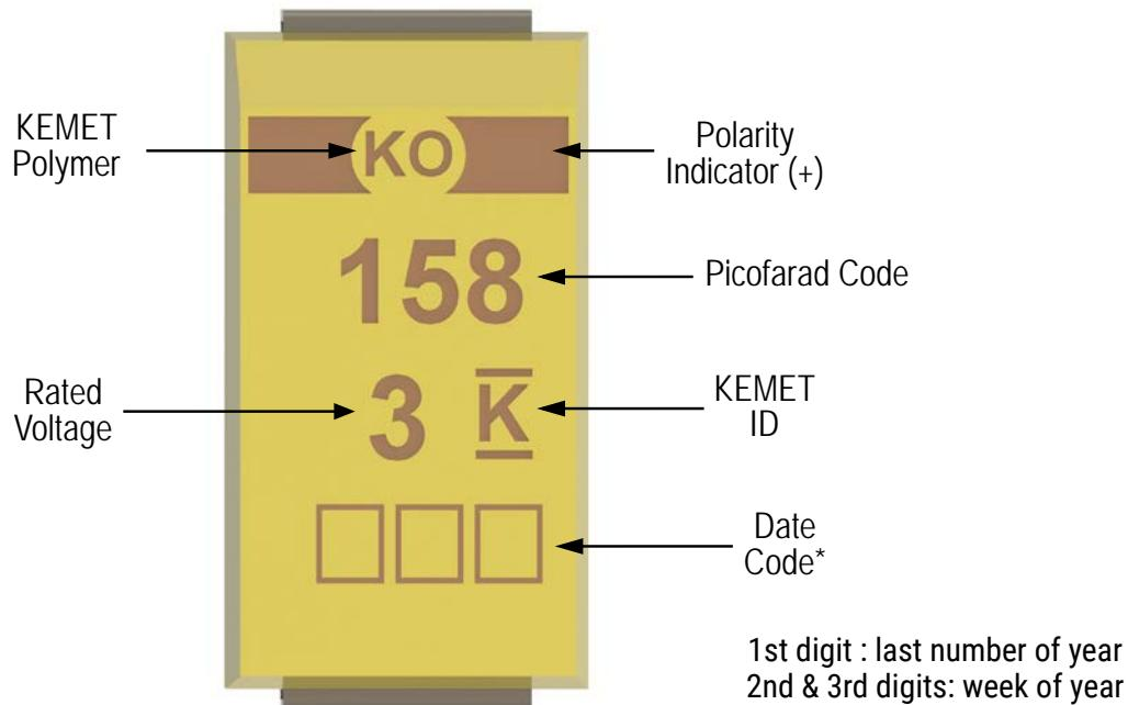
*Note: The marking observed is for the discrete capacitor used in the construction of the stacked product*
