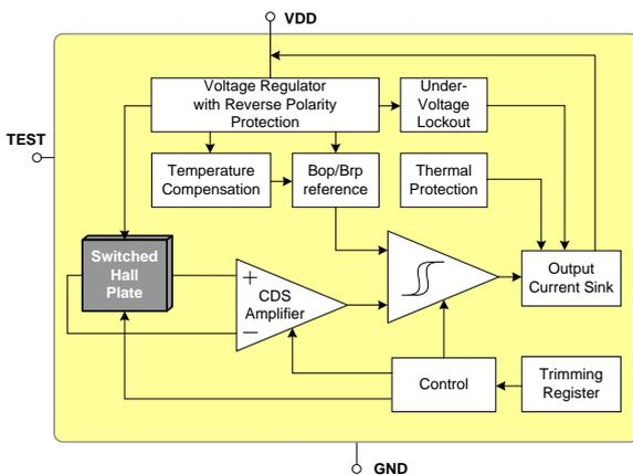
The included voltage regulator operates from 2.7 to 24V, hence covering a wide range of applications. With the built-in reverse voltage protection, a serial resistor or diode on the supply line is not required so that even remote sensors can be specified for low voltage operation down to 2.7V while being reverse voltage tolerant.
