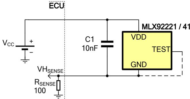
1. For proper operation, a 10nF bypass should be placed as close as possible to the  $V_{DD}$  and ground.
