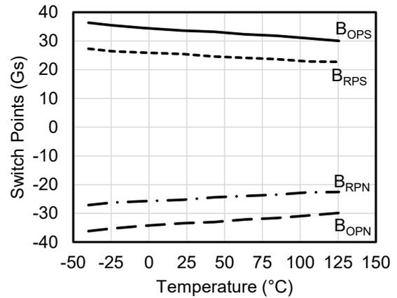
Figure 12. Switch points versus temperature ( $V_{CC} = 3\text{ V}$ )
