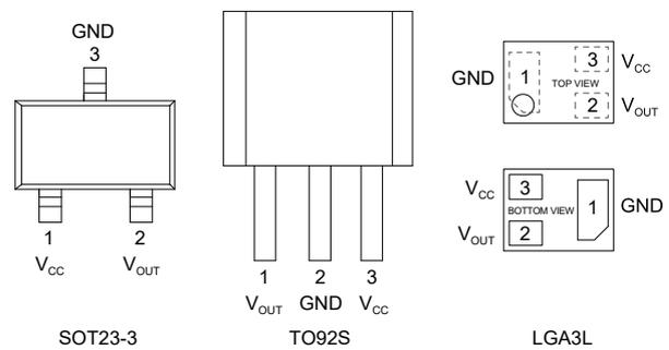
Figure 4. Pin configuration
