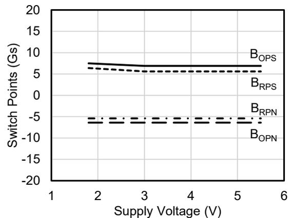
Figure 9. Switch points versus supply voltage (T<sub>A</sub>=25°C)
