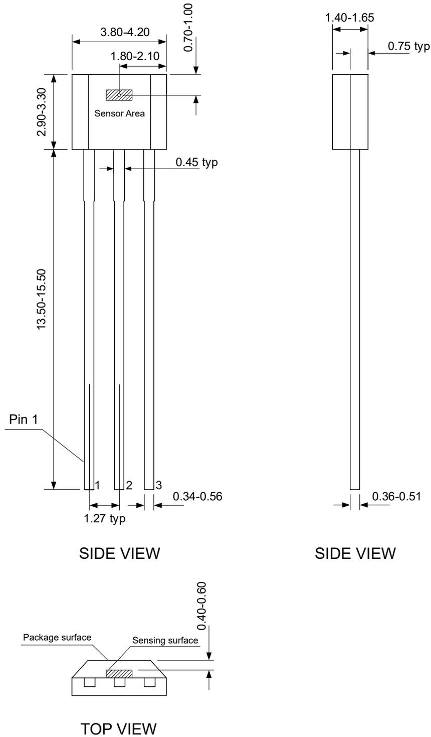
Figure 18. Package outline of TO92S (unit: mm)
