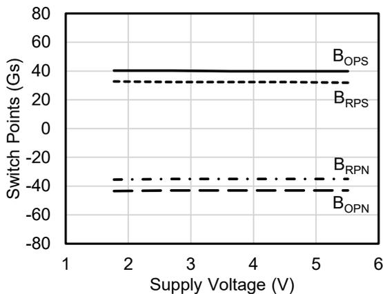
Figure 8. Switch points versus supply voltage (T<sub>A</sub>=25°C)
