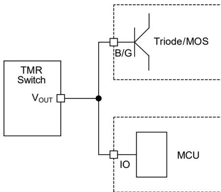
Figure 16. Application diagram for driving power load
