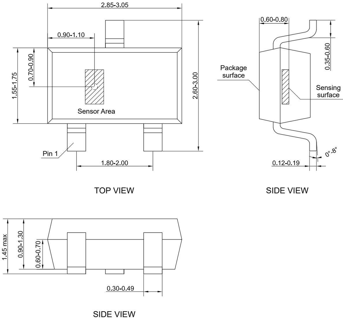
Figure 17. Package outline of SOT23-3 (unit: mm)
