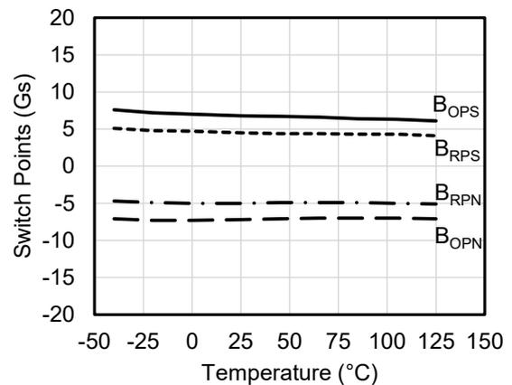
Figure 14. Switch points versus temperature ( $V_{CC} = 3\text{ V}$ )
