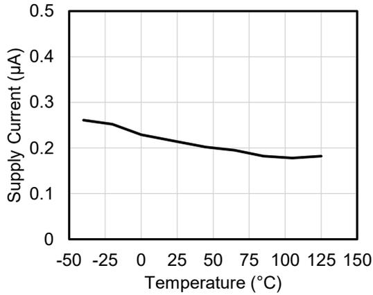
Figure 10. Supply current versus temperature ( $V_{CC} = 3\text{ V}$ )
