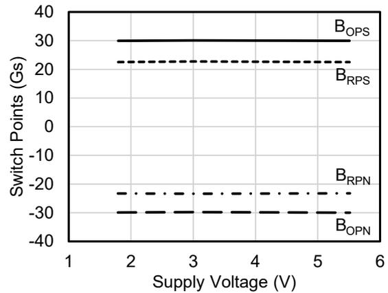
Figure 7. Switch points versus supply voltage (T<sub>A</sub>=25°C)
