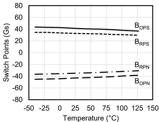
Figure 13. Switch points versus temperature ( $V_{CC} = 3\text{ V}$ )
