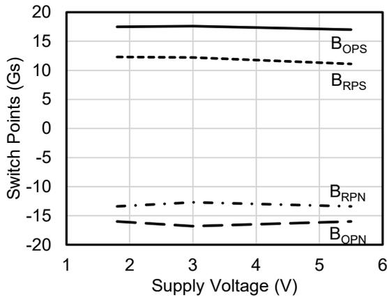
Figure 6. Switch points versus supply voltage (T<sub>A</sub>=25°C)
