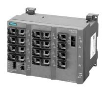
SCALANCE X320-1FE managed IE switch, 20x 10/100 Mbit/s RJ45 ports, 1x 100 Mbit/s SC Port multimode LED-diagnostics, error-signaling contact with Select/set pushbutton, PROFINET IO Device, network management, integrated redundancy manager, Office features (RSTP, VLAN, IGMP,...) C-plug in scope of delivery .
