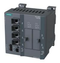
SCALANCE X308-2M; managed IE switch, compact; 4x 10/100/1000 Mbit/s for RJ45 ports electrical; 2x 100/1000 Mbit/s for 2-port media modules, electrical or optical; LED diagnostics; error signaling contact; select/set pushbutton; PROFINET IO device; network management; Integrated redundancy manager; office features (RSTP, VLAN, IGMP,..); C-PLUG in scope of supply.
