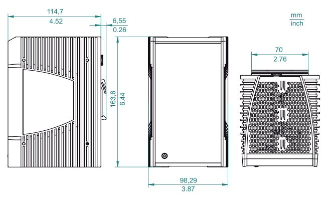
Figure 11: Dimensions of device variants with operating temperature characteristic value E and T. For the characteristic value, cf. "Device name and product code" on page 24.
