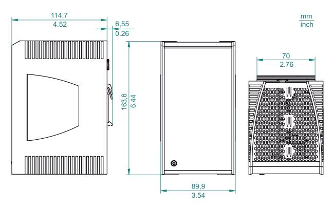
Figure 10: Dimensions of the device variants with operating temperature characteristic value S. For the characteristic value, cf. "Device name and product code" on page 24.
