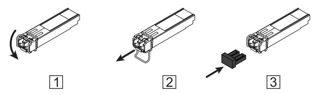
Figure 9: De-installing SFP transceivers: De-installation sequence
