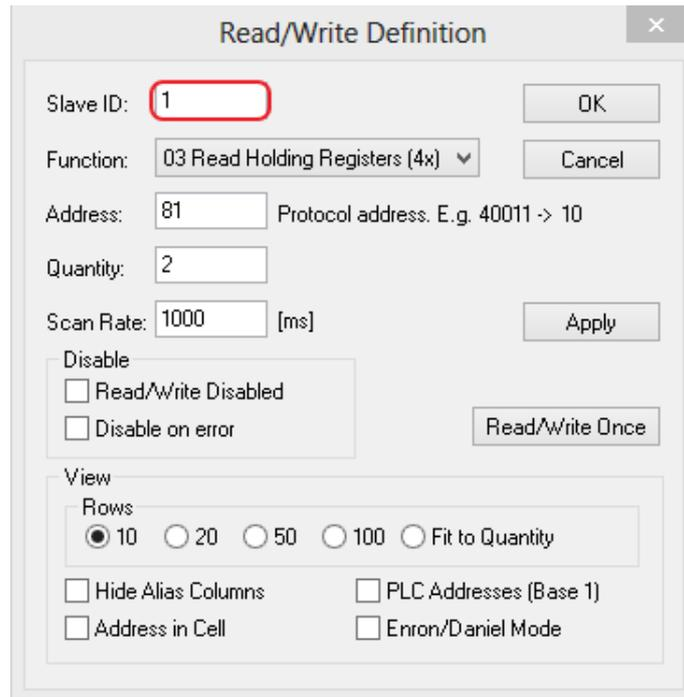
Figure 2.34 Slave ID in the Modbus Poll Function is set to 1
