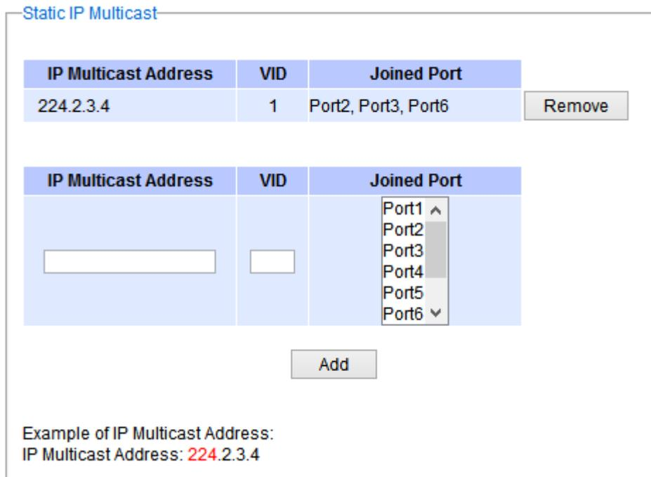
Figure 2.90 Example of Static IP Multicast Setting
