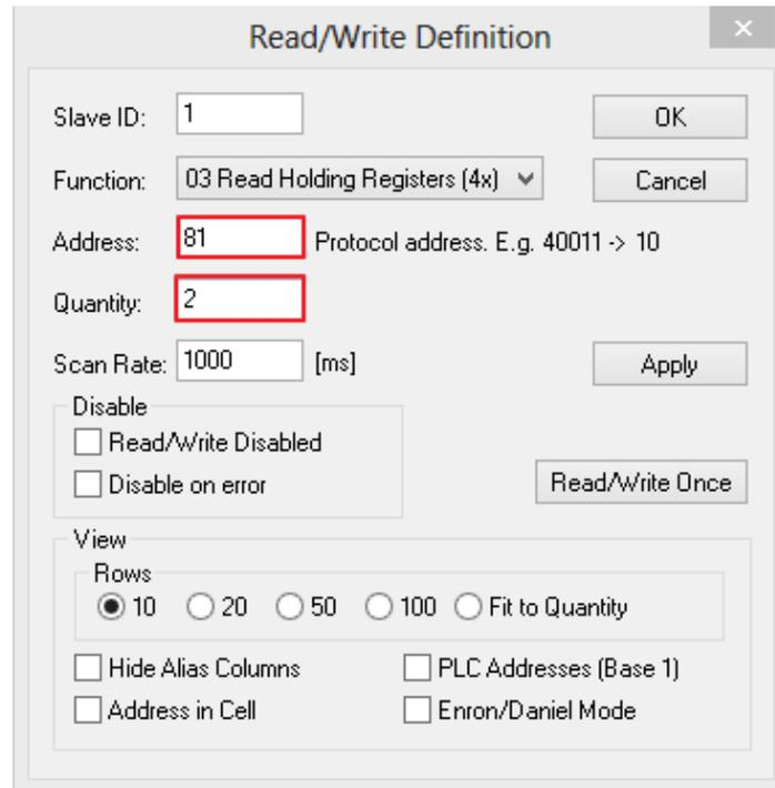
Figure 2.36 Setup Starting Address and Quantity in Modbus Poll
