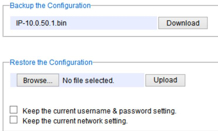
Figure 2.170 Backup/Restore Configuration via HTTP
