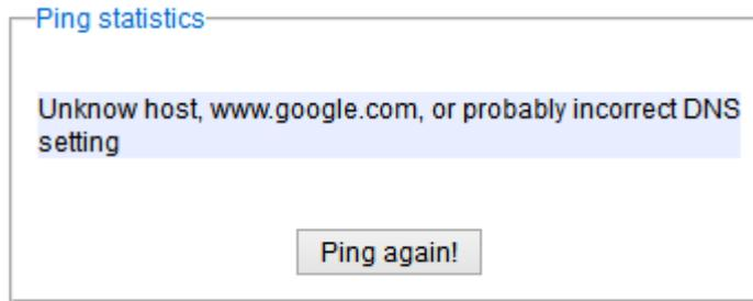
Figure 2.22 Example of unsuccessful ping command result
