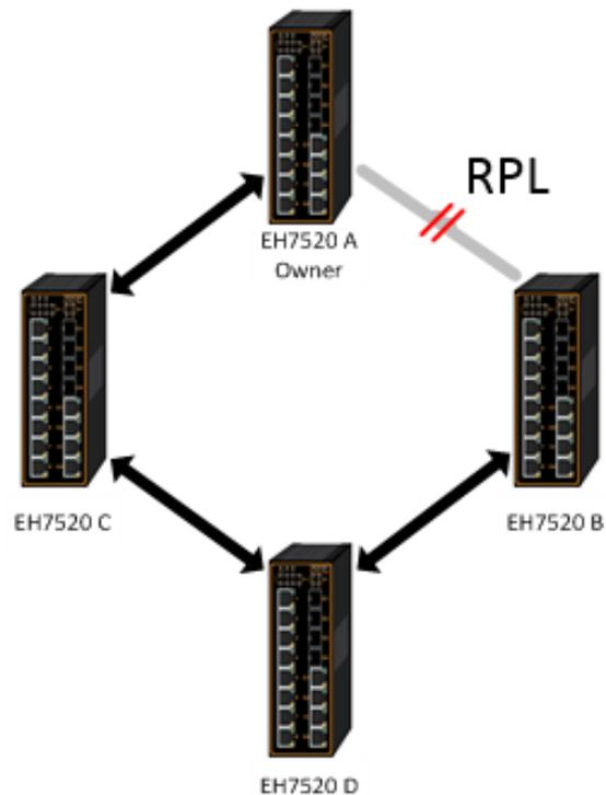
Figure 2.128 An Example of Ring Topology (Example made on EH7520)
