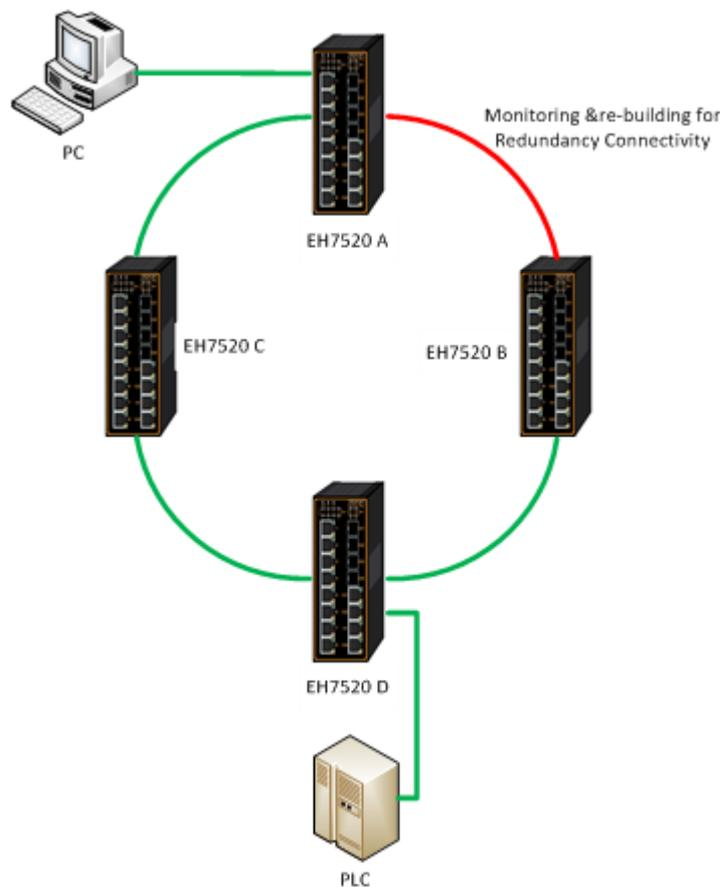
Figure 2.137 iA-Ring Example Topology (Example made on EH7520)
