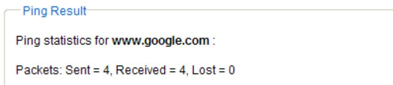
Figure 2.21 Example of successful ping command result
