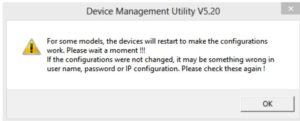
Figure 5.7 Warning Dialog before the Device Restart
