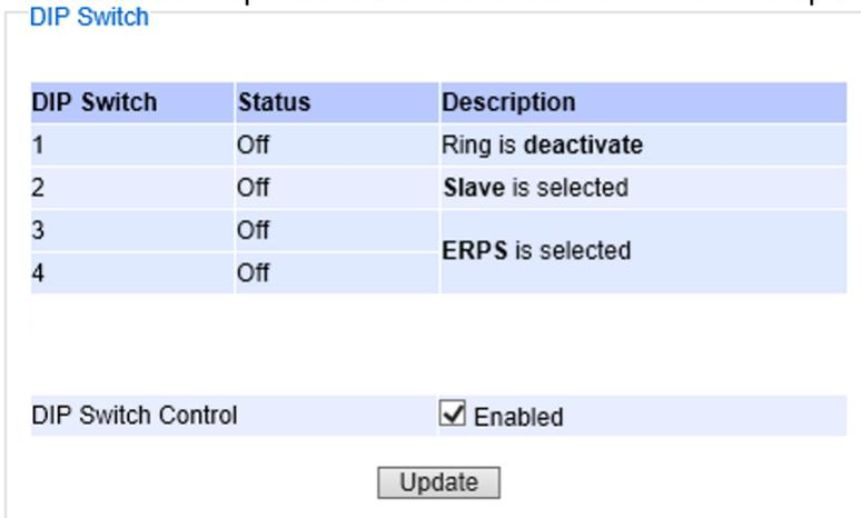
Figure 2.48 shows the DIP switch webpage. The bottom portion allows the users to enable or disable the physical control of the DIP Switch by checking on the **DIP Switch Control** option. This is another easy and convenient way to configure ERPS or iA-ring or Compatible-Ring using the DIP Switches instead of modifying configuration on a web browser. After checking or unchecking the option, please click **Update** button to allow the setting to take effect on the managed switch.
