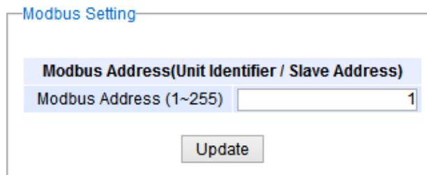
Figure 2.27 Webpage for Setting the Modbus Address
