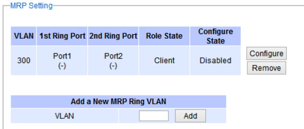
Figure 2.152 Example of PROFINET's MRP VLAN Entry
