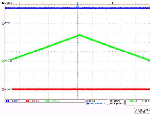
$V_{SENSE}$  ramp from 0 V to 1.4V,  $V_{DD} = 3.3$  V,  $V_{CT} = 0$  V
