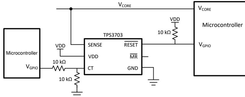
Figure 9-11. Window Voltage Monitoring with  $\overline{\text{RESET}}$  Latch
