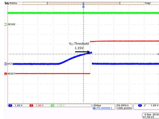
$V_{CT}$  biased at least to 1.15 V,  $V_{SENSE} = 1.2$  V
