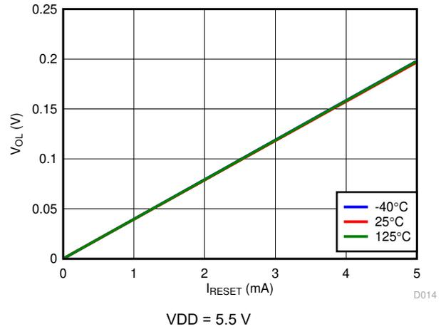
**Figure 7-16. Low-Level Output Voltage vs RESET current**
