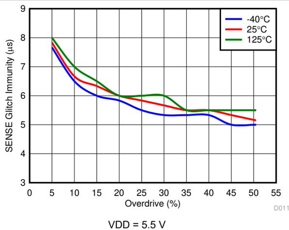
Figure 7-13. SENSE Glitch Immunity ( $V_{IT-}$ ) vs Overdrive
