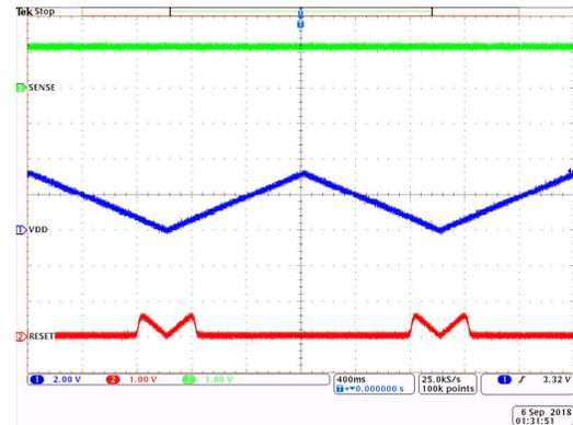
$V_{DD}$  ramp up from 0 V to 3.3 V,  $V_{SENSE} = 1.2$  V, CT = 0 V
