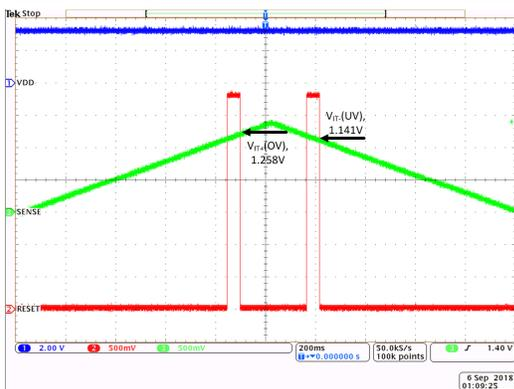
$V_{SENSE}$  ramp from 0 V to 1.4 V,  $V_{DD} = 3.3$  V, CT = OPEN
