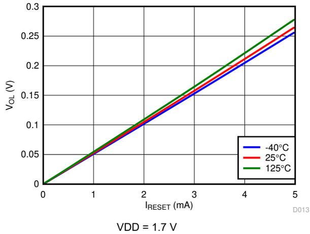
**Figure 7-15. Low-Level Output Voltage vs RESET current**
