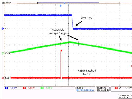
$V_{Sense}$  ramp from 0 V to 1.4 V,  $V_{DD} = 3.3$  V,  $V_{RESET} = V_{DD}$
