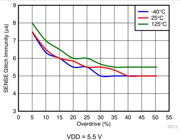
Figure 7-14. SENSE Glitch Immunity ( $V_{IT+}$ ) vs Overdrive
