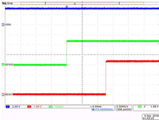
$V_{SENSE}$  Start up from 0 V to 1.2 V,  $V_{DD} = 3.3$  V, CT = OPEN
