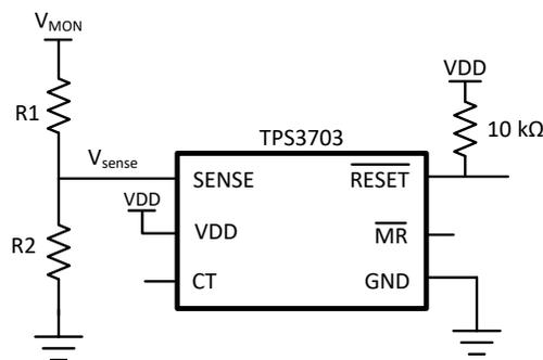
Figure 9-4. Adjustable Voltage Threshold with External Resistor Dividers
