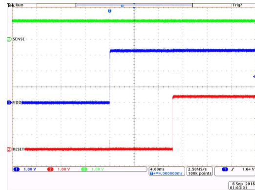
$V_{DD}$  Start up from 0 V to 3.3 V,  $V_{SENSE} = 1.2$  V, CT = OPEN
