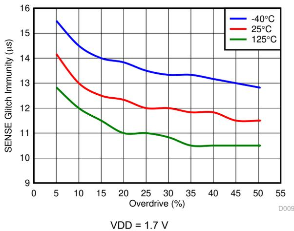
Figure 7-11. SENSE Glitch Immunity ( $V_{IT-}$ ) vs Overdrive
