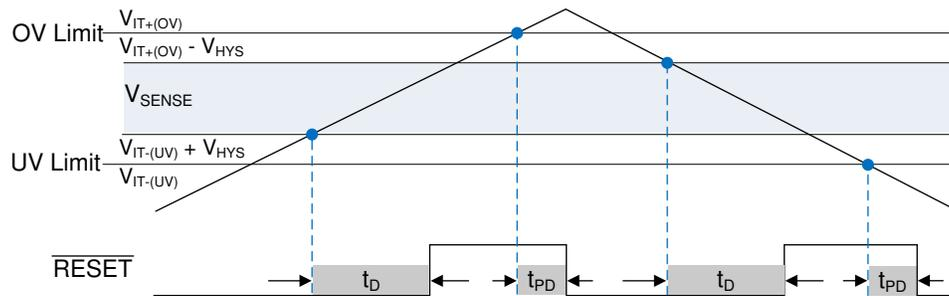
Figure 8-1. RESET output
