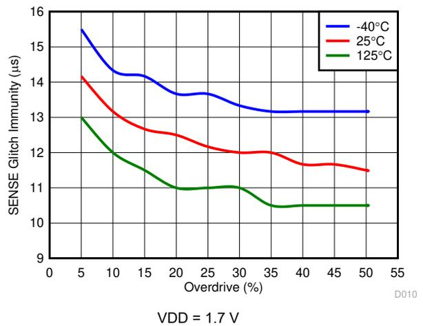
Figure 7-12. SENSE Glitch Immunity ( $V_{IT+}$ ) vs Overdrive
