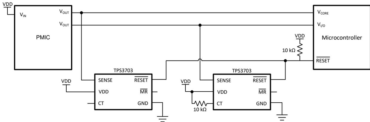
Figure 9-6. Two TPS3703 Monitoring Two Microcontroller Power Rails
