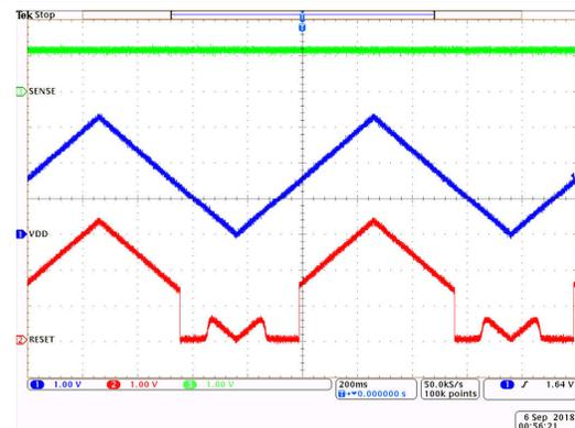
$V_{DD}$  ramp from 0 V to 3.3 V,  $V_{SENSE} = 1.2$  V, CT = OPEN
