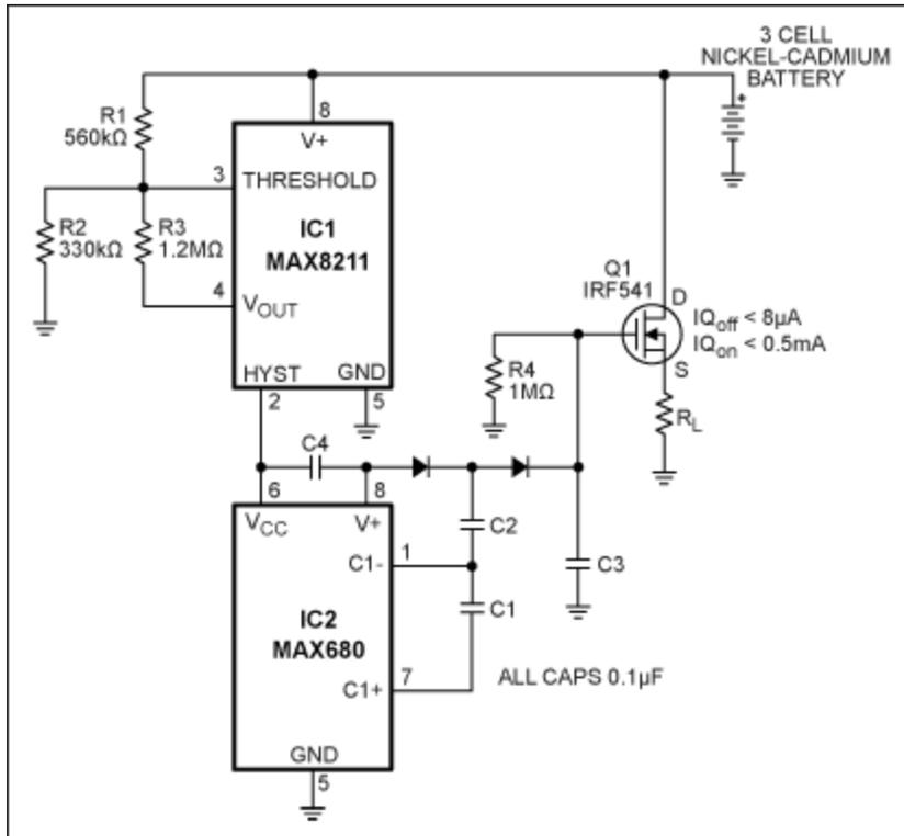
Figure 1. When battery voltage drops below a threshold set by R1 and R2, the voltage-detector chip (IC1) removes power from the charge pump IC2, which turns off the high-side switch Q1 by removing its gate drive.
