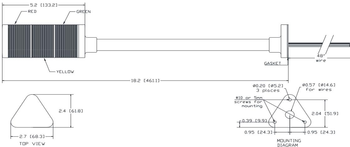
**LED OPERATION:** CONNECT STACK COLOR WIRE TO POWER AND BROWN WIRE TO POWER.
