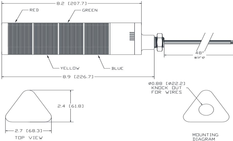
**LED OPERATION:** CONNECT STACK COLOR WIRE TO POWER AND BROWN WIRE TO POWER.
