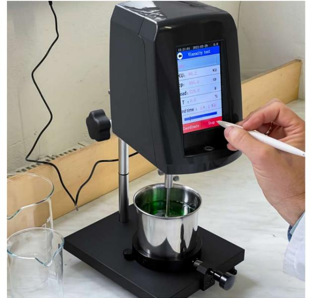
**Viscometer / viscosity meter with PC interface / Optional ISO factory certificate / Touchscreen /
