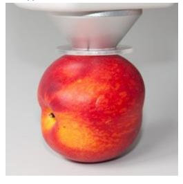
Here you can see the Colorimeter PCE-CSM 2 in progress. Due to the 8 mm measurement aperture the device is also designed for smaller surfaces. Especially for food the device is very handy, since only the measuring aperture covers the surface of the measured object instead of the whole measurement device like with other measuring devices.
