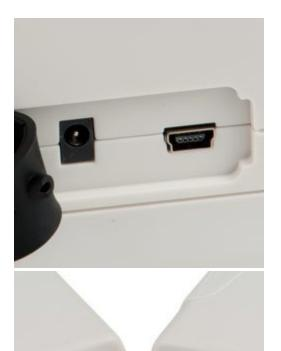
Here you can see the inputs at the colourimeter PCE-CSM 2 and PCE-CSM 4. One of these is compatible with the adapter for recharging the device's battery (in image left input). The other one is a RS232 interface for USB connections to a computer or printer, in order to evaluate the data by means of the software included in delivery.
