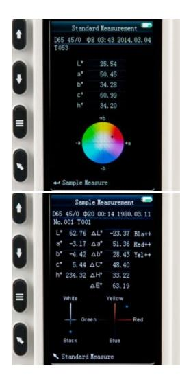
Here you can see the user interface of the Colorimeter PCE-CSM 2 and PCE-CSM 4 during standard measurements. That interface starts as soon as the device initiates the measuring process. The Colorimeter does not only display the various values of the parameter, but it also illustrates the measuring results in a graphic as you can see here.
