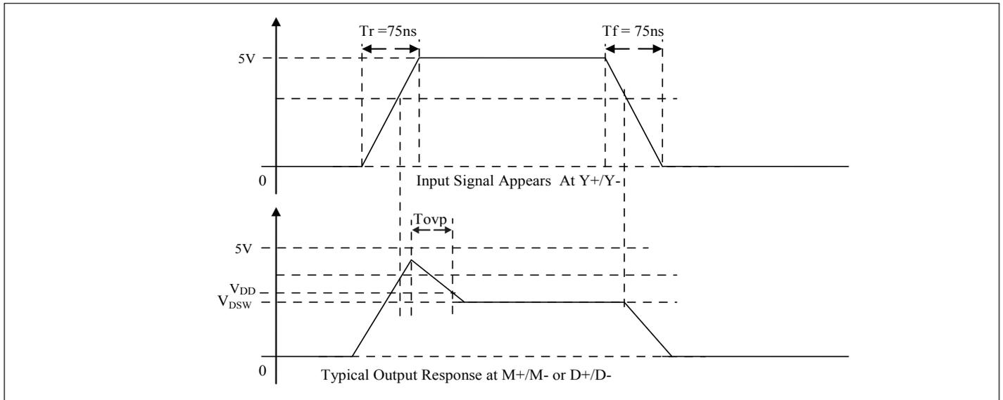
The PI3USB102J offers overvoltage protection for the I/O pins to protect from shorts to VBUS (5V). When a 5V is applied to Y+/Y-, the voltage at M+/M-, and D+/D- falls to 3.6V within the time  $T_{OVP}$  then clamps to  $V_{DSW}$ .
