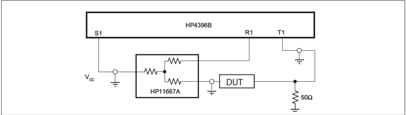
**Test Circuit for Electrical Characteristics**
