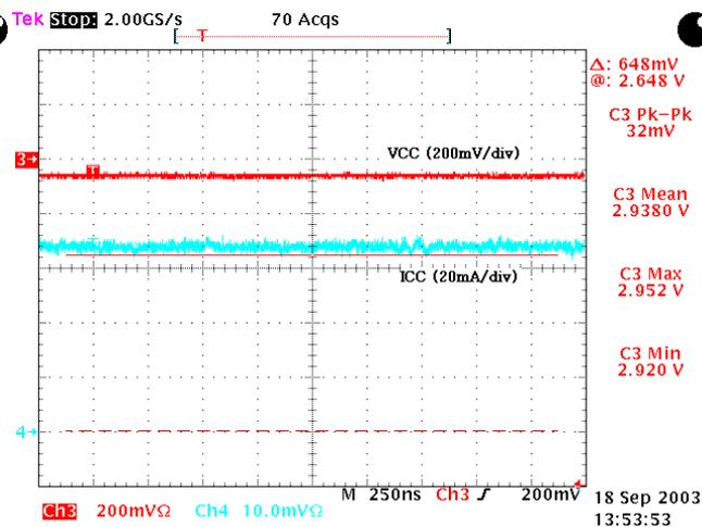
**Figure 3-3: C11 (3V) w/65mA dc load current**
