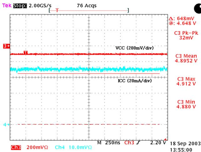
**Figure 3-2: C11 (5V) w/65mA dc load current**
