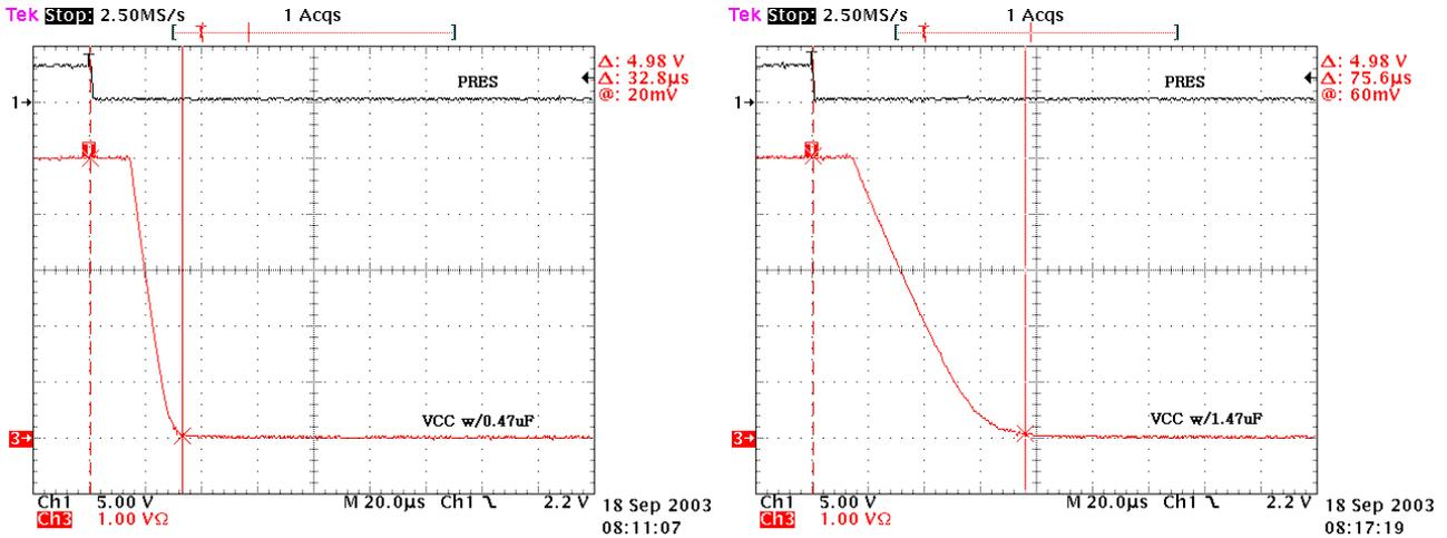
**Figure 3-4: Deactivation time ( $0.47\mu F @V_{CC}$ )** **Figure 3-5: Deactivation time ( $1.47\mu F @V_{CC}$ )**
