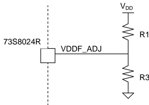
Figure 3-6: External resistor divider for setting  $V_{DDTH}$
