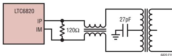
**Figure 19. Connection of Transformer and Common Mode Choke**
