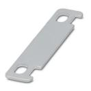
Cable marker, Aluminum label, aluminum color, unlabeled, can be labeled with: BLUEMARK ID COLOR, BLUEMARK ID, BLUEMARK CLED, mounting type: Assembly with cable ties, cable diameter: > 2.9 mm, lettering field size: 29 x 8 mm
