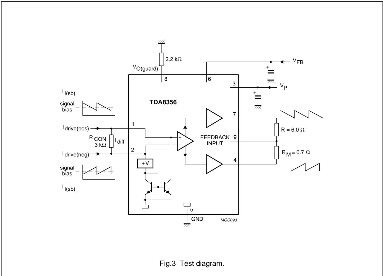
Fig.3 Test diagram.
