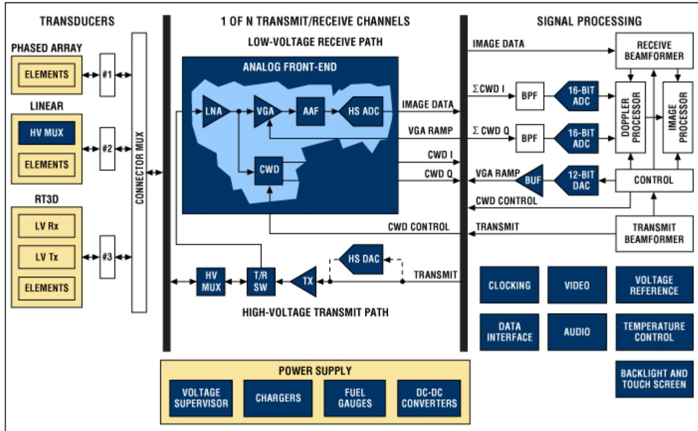
Functional block diagram of an ultrasound imaging system. For a list of Maxim's recommended ultrasound solutions, please go to: [www.maximintegrated.com/ultrasound](http://www.maximintegrated.com/ultrasound).
