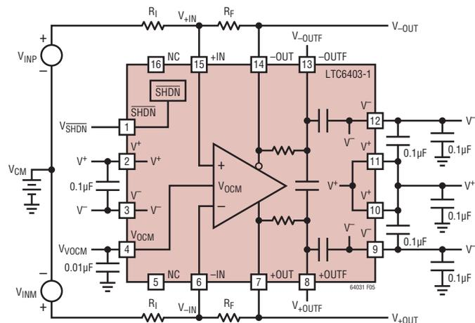
Figure 5. Circuit for Common Mode Range
