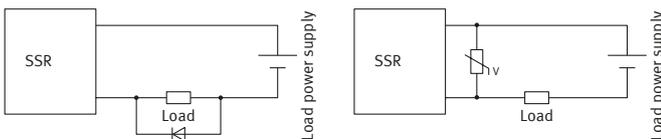
3) Clamp diode and snubber circuit can limit spike voltages at the load side. However, long wires may cause spike voltages due to inductance. It is recommended to keep wires as short as possible to minimize inductance.
