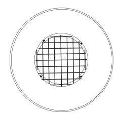
2) Once screen is in place, attach duct back onto nozzle.
