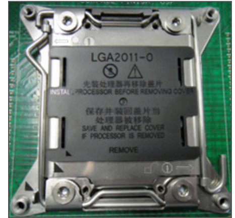
LGA 2011-0 CPU Socket with Standard Independent Loading Mechanism (ILM) and (optional) ILM cover
