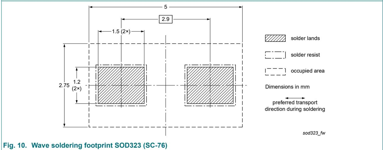
Fig. 10. Wave soldering footprint SOD323 (SC-76)
