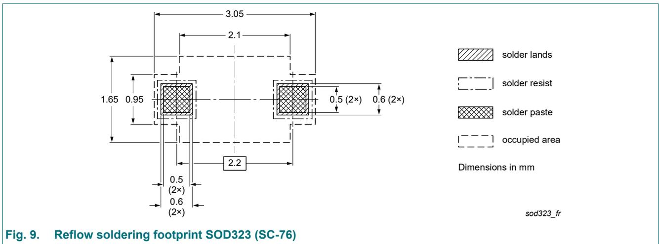
Fig. 9. Reflow soldering footprint SOD323 (SC-76)
