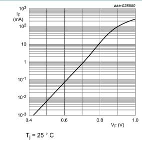
Fig. 1. Forward current as a function of forward voltage; typical values (MM5Z2V4T5G)
