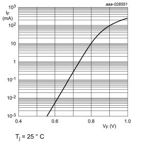
Fig. 2. Forward current as a function of forward voltage; typical values (MM5Z6V8T5G)
