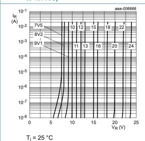
Fig. 7. Reverse current as a function of reverse voltage; typical values (MM5Z7V5T5G to 24VT5G)
