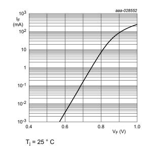
Fig. 3. Forward current as a function of forward voltage; typical values (MM5Z7V5T5G)
