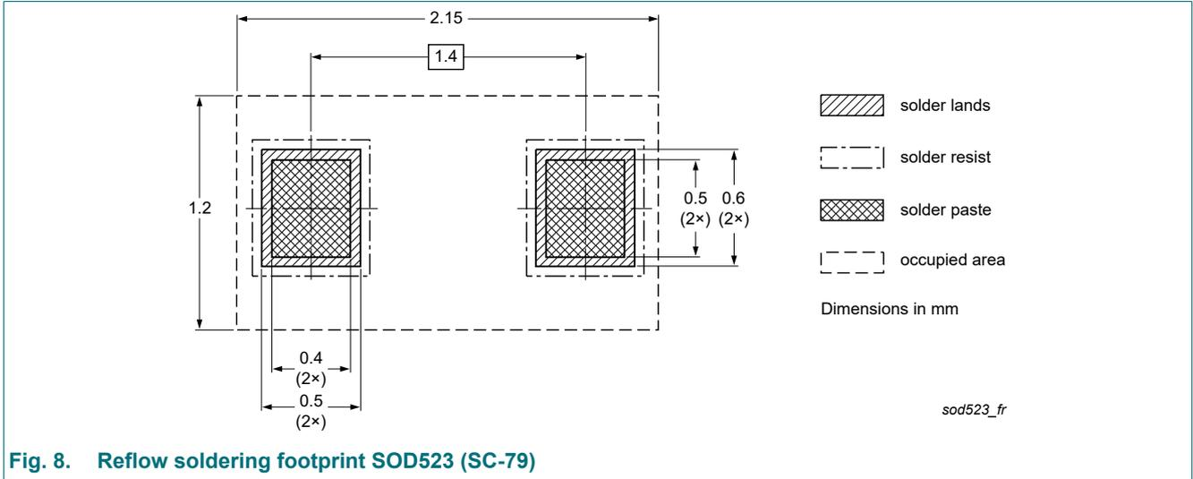
**Fig. 8. Reflow soldering footprint SOD523 (SC-79)**
