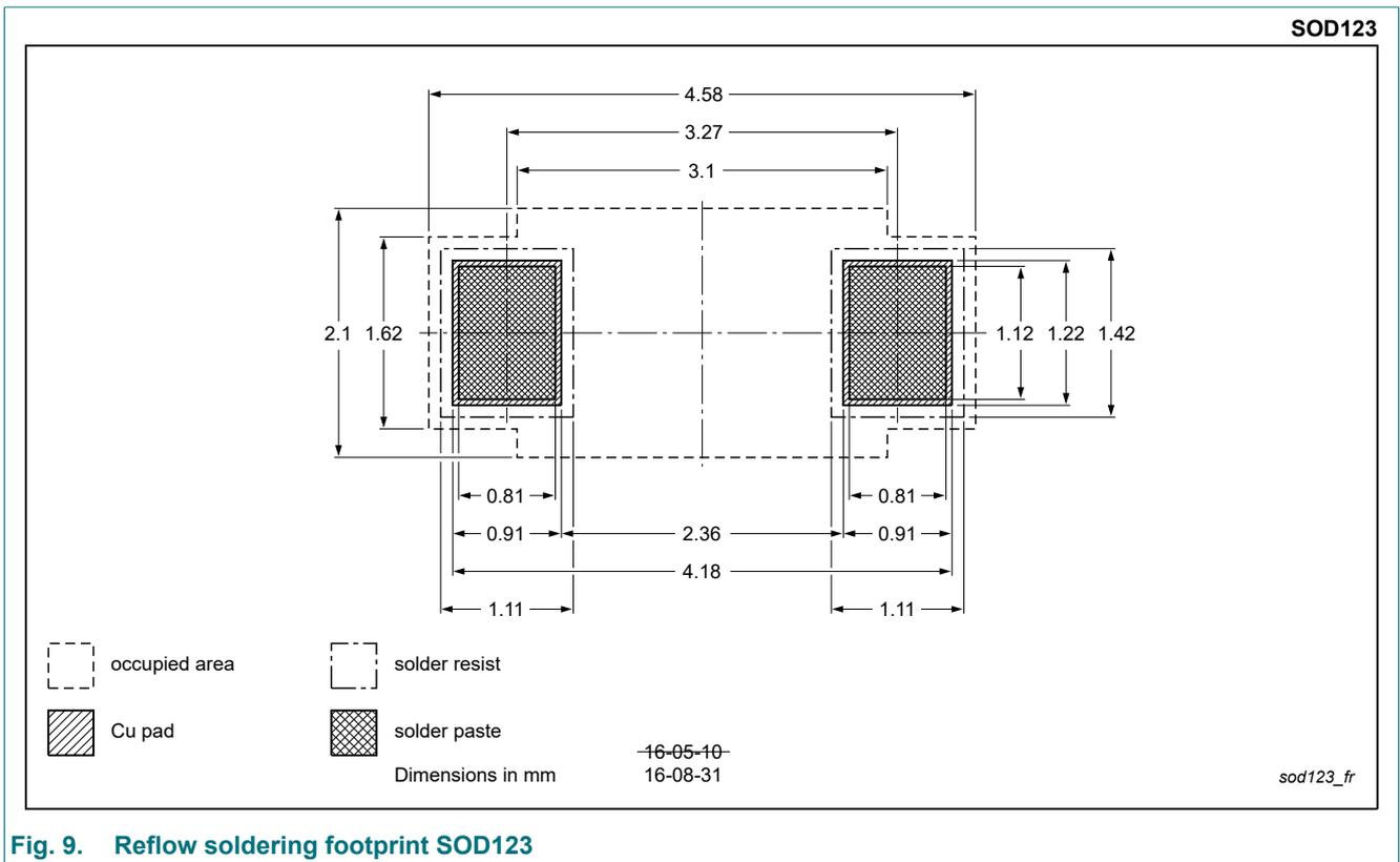
Fig. 9. Reflow soldering footprint SOD123
