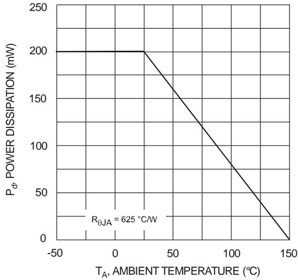
Fig. 1 Derating Curve
