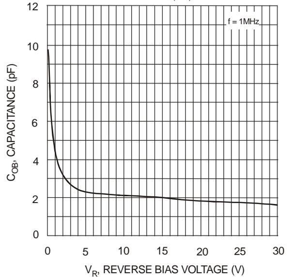
Fig. 4 Output Capacitance
