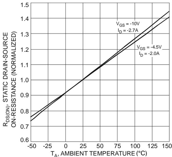
Fig. 5 Normalized Static Drain-Source On-Resistance vs. Ambient Temperature
