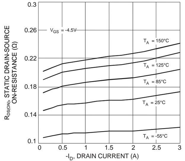
Fig. 4 On-Resistance vs. Drain Current and Gate Voltage
