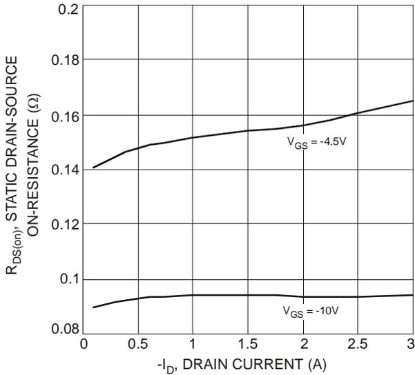
Fig. 3 On-Resistance vs. Drain Current and Gate Voltage
