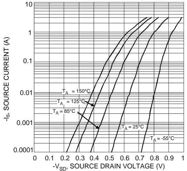
Fig. 8 Reverse Source Current vs. Source-Drain Voltage
