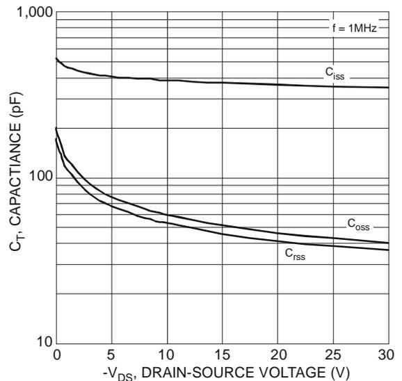
Fig. 6 Typical Capacitance
