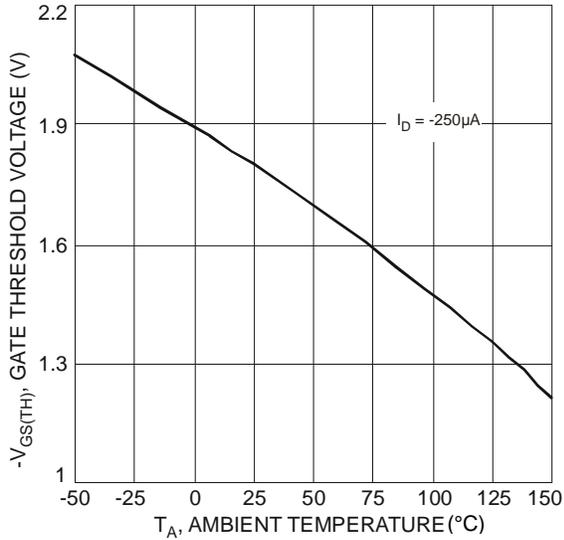
Fig. 7 Gate Threshold Voltage vs. Ambient Temperature
