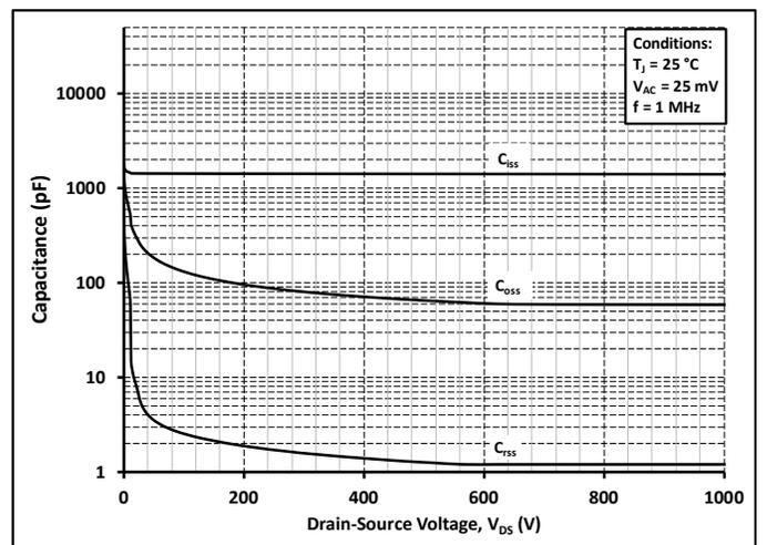
Figure 18. Capacitances vs. Drain-Source Voltage (0 - 1000V)
