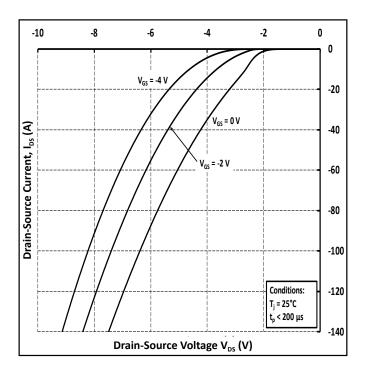
Figure 9. Body Diode Characteristic at 25 °C
