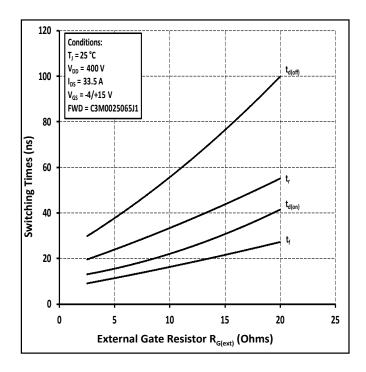
Figure 26. Switching Times vs  $R_{\text{G(ext)}}$
