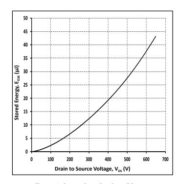
Figure 16. Output Capacitor Stored Energy
