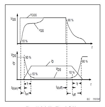
Figure 27. Switching Times Definition
