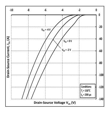
Figure 10. Body Diode Characteristic at 150 °C
