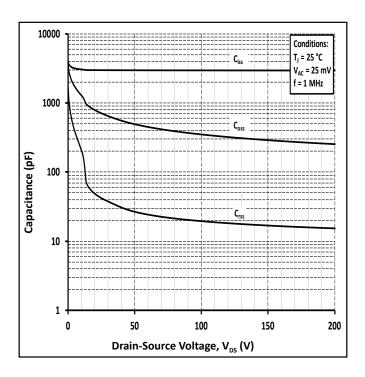
Figure 17. Capacitances vs Drain-Source Voltage (0-200 V)
