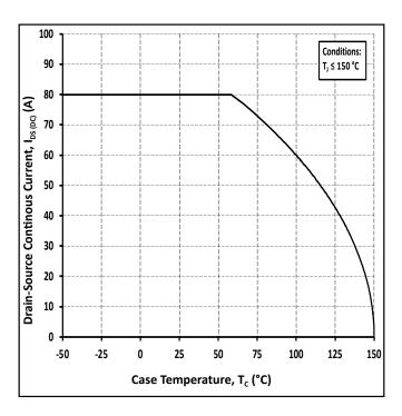
Figure 19. Continuous Drain Current Derating vs Case Temperature
