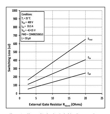
Figure 24. Clamped Inductive Switching Energy vs R<sub>G(ext)</sub>
