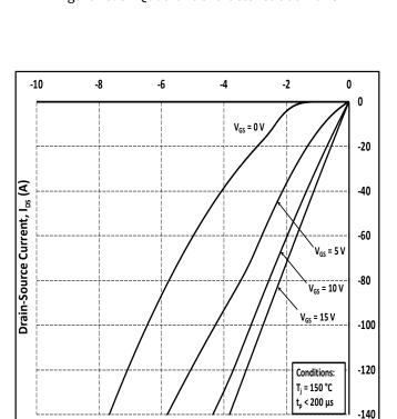
Figure 15. 3<sup>rd</sup> Quadrant Characteristic at 150 °C
