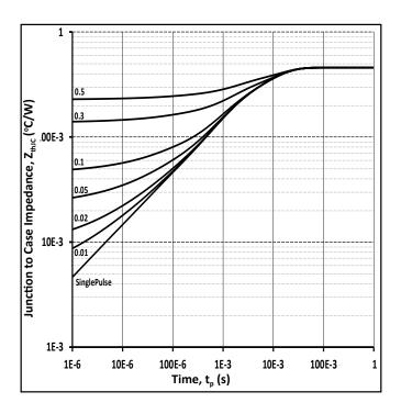
Figure 21. Transient Thermal Impedance (Junction - Case)
