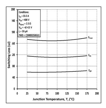
Figure 25. Clamped Inductive Switching Energy vs Temperature
