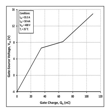
Figure 12. Gate Charge Characteristic
