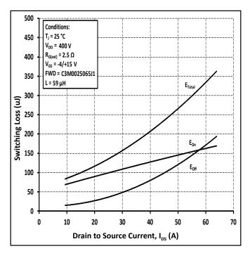
Figure 23. Clamped Inductive Switching Energy vs Drain Current ( $V_{DD}$  = 400 V)
