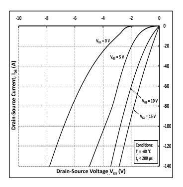
Figure 13. 3<sup>rd</sup> Quadrant Characteristic at -40 °C
