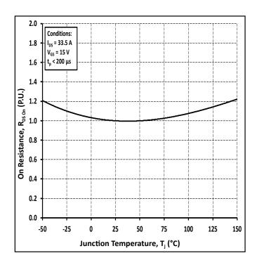
Figure 4. Normalized On-Resistance vs Temperature
