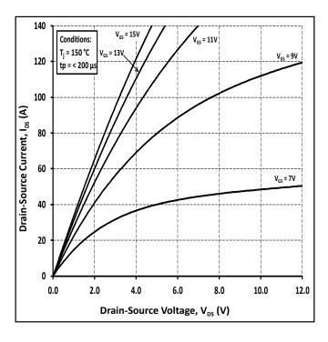
Figure 3. Output Characteristics T<sub>J</sub> = 150 °C
