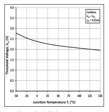
Figure 11. Threshold Voltage vs Temperature
