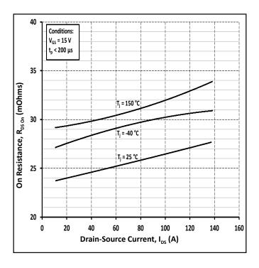
Figure 5. On-Resistance vs Drain Current for Various Temperatures
