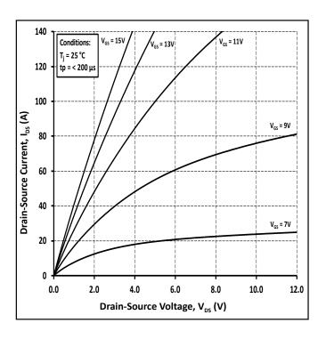
Figure 2. Output Characteristics  $T_1 = 25$  °C
