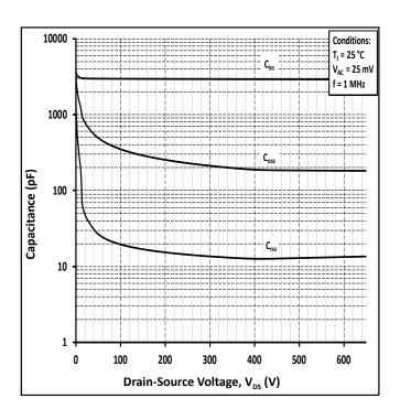
Figure 18. Capacitances vs Drain-Source Voltage (0-600 V)
