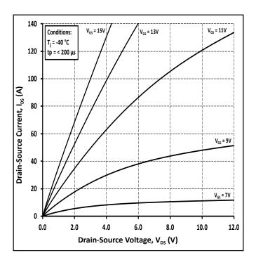
Figure 1. Output Characteristics T<sub>1</sub> = -40 °C
