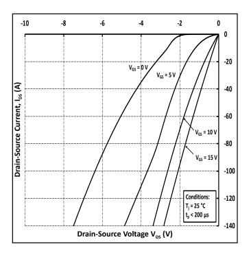
Figure 14. 3<sup>rd</sup> Quadrant Characteristic at 25 °C
