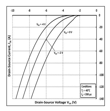
Figure 8. Body Diode Characteristic at -40 °C
