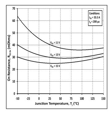
Figure 6. On-Resistance vs Temperature for Various Gate Voltage
