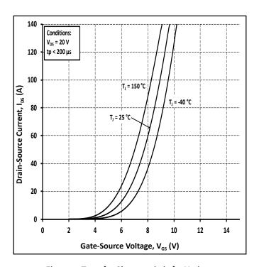
Figure 7. Transfer Characteristic for Various Junction Temperatures
