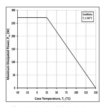
Figure 20. Maximum Power Dissipation Derating vs Case Temperature
