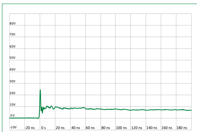
ISO10605 Contact Discharge Plot at +8 kV
