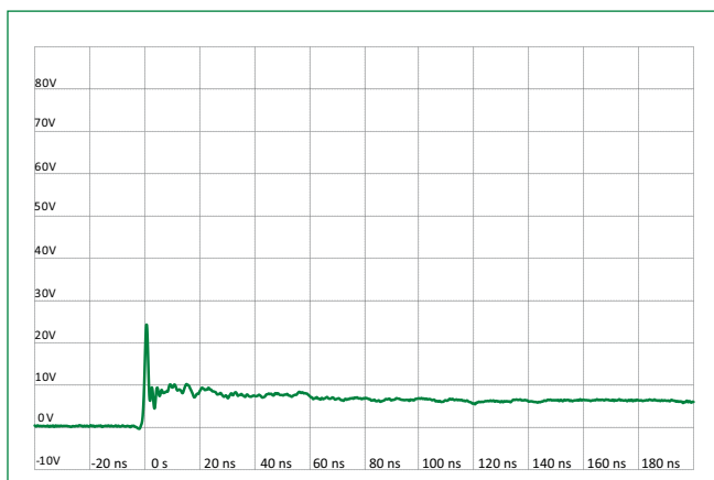
IEC 61000-4-2 +8 kV Contact ESD Clamping Voltage
