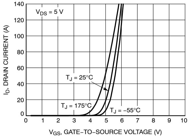
Figure 2. Transfer Characteristics
