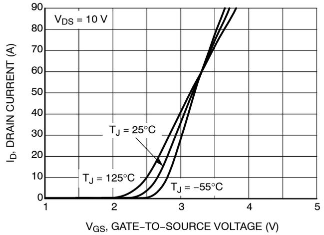
Figure 2. Transfer Characteristics
