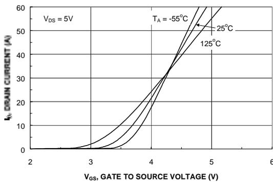
**Figure 5. Transfer Characteristics.**
