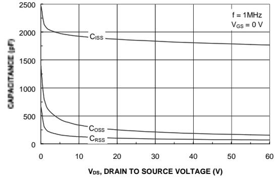
**Figure 8. Capacitance Characteristics.**
