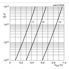
$$T_j = 25 \, ^{\circ}C; \, V_{DS} = -5 \, V$$
