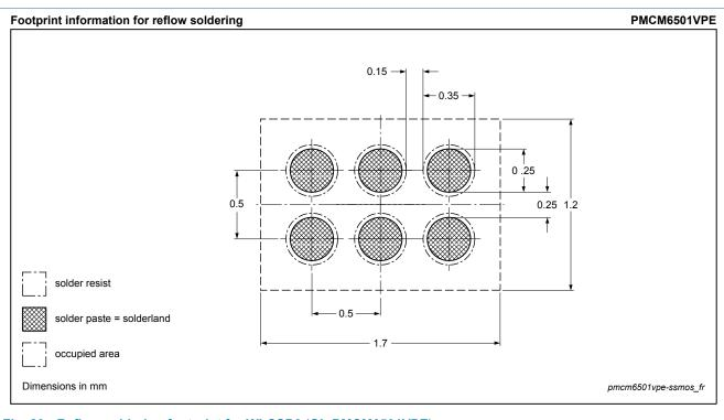
Fig. 20. Reflow soldering footprint for WLCSP6 (OL-PMCM6501VPE)
