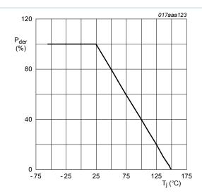
Fig. 2. MOSFET transistor: Normalized total power dissipation as a function of junction temperature
