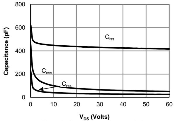
**Figure 8: Capacitance Characteristics**
