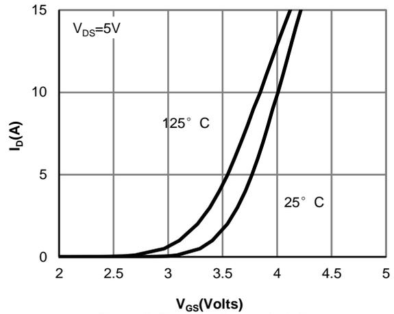
**Figure 2: Transfer Characteristics**
