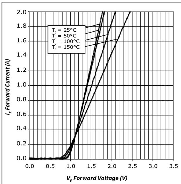
Figure 1. Forward Characteristics
