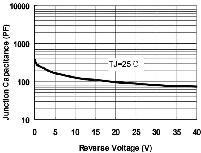
Fig.1-Typical Junction Capacitance
