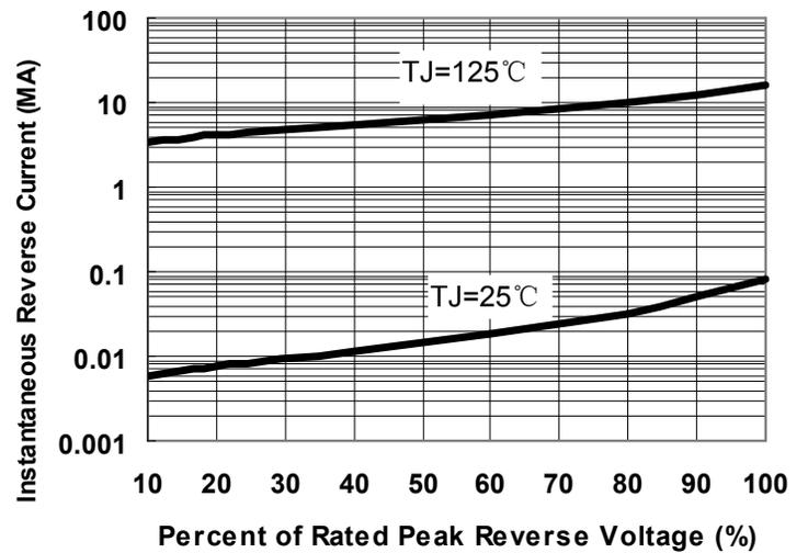
Fig.2-Typical Reverse Current
