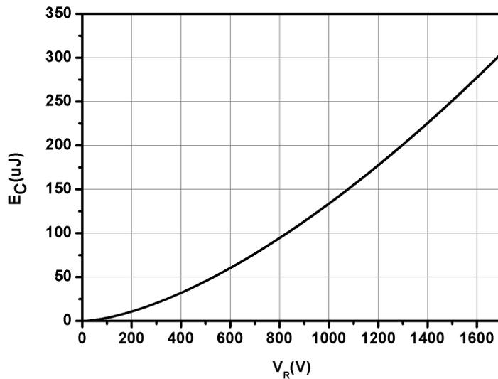
Fig.7-Capacitance Stored Energy
