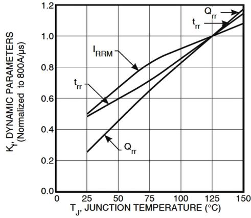
Figure 6 • Dynamic Parameters vs. Junction Temperature
