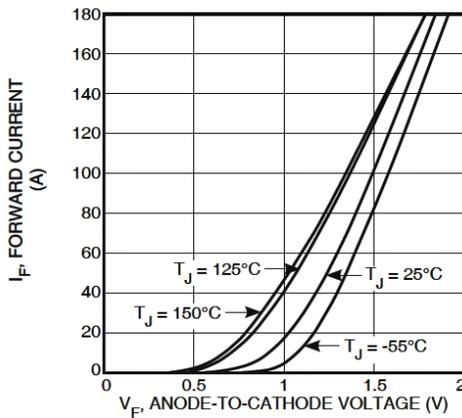
Figure 2 • Forward Current vs. Forward Voltage
