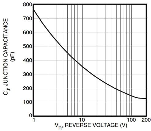
Figure 8 • Junction Capacitance vs. Reverse Voltage
