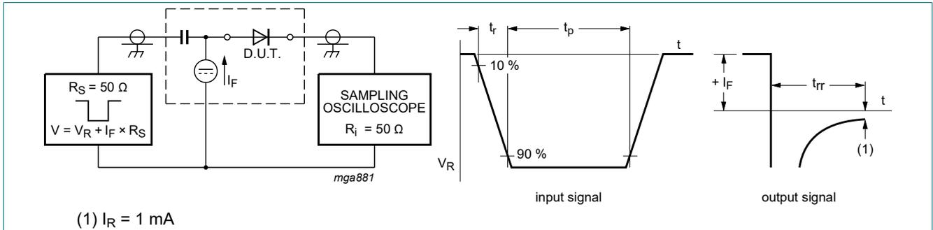
Fig. 6. Reverse recovery time test circuit and waveforms
