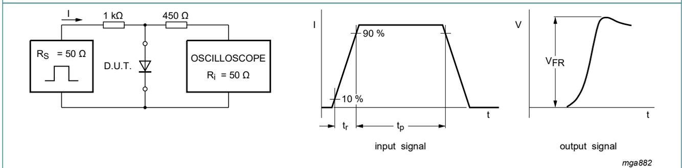
Fig. 7. Forward recovery voltage test circuit and waveforms
