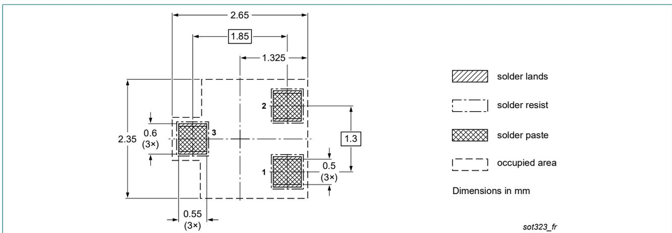
Fig. 8. Reflow soldering footprint for SC-70 (SOT323)
