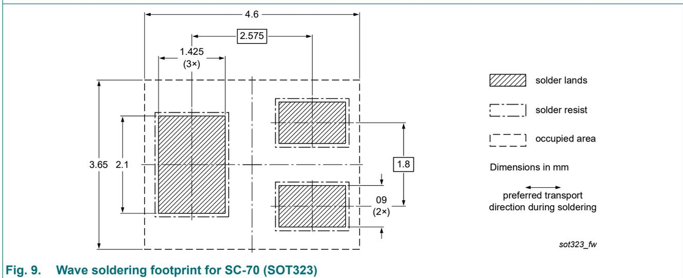
Fig. 9. Wave soldering footprint for SC-70 (SOT323)
