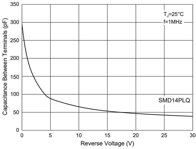
Fig. 8 - Capacitance Characteristics
