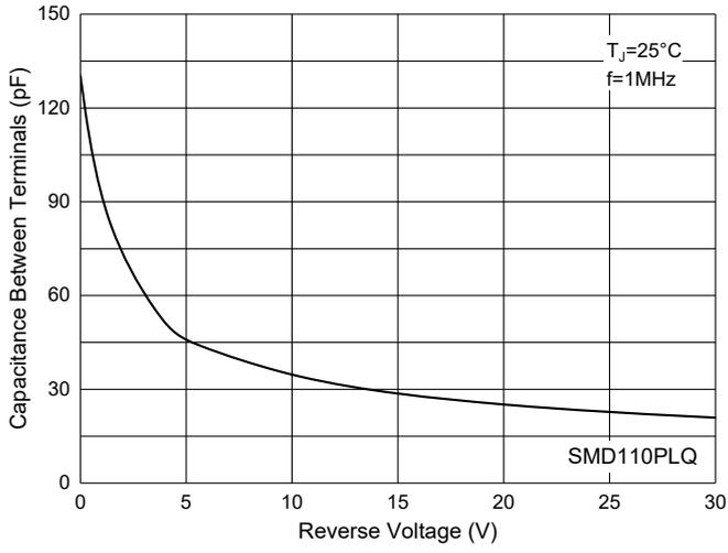
Fig. 8 - Capacitance Characteristics
