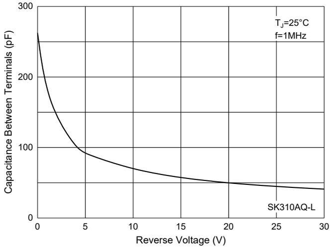
Fig. 8 - Capacitance Characteristics
