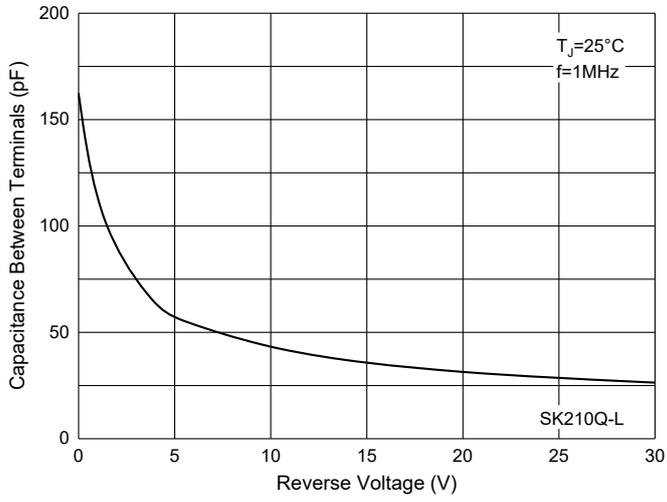
Fig. 8 - Capacitance Characteristics
