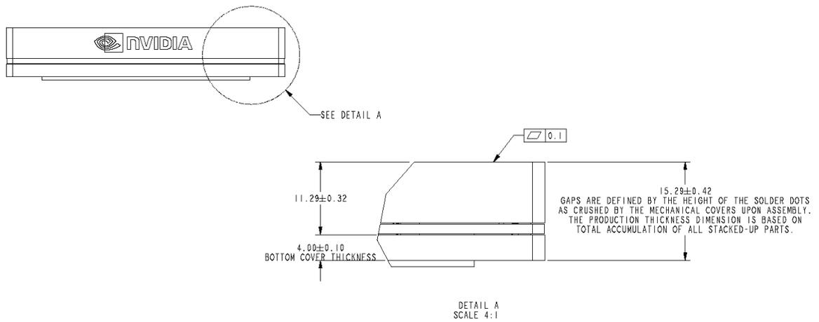
Figure 7-4. Module Mechanical Drawing - Midpoint of the Connector View
