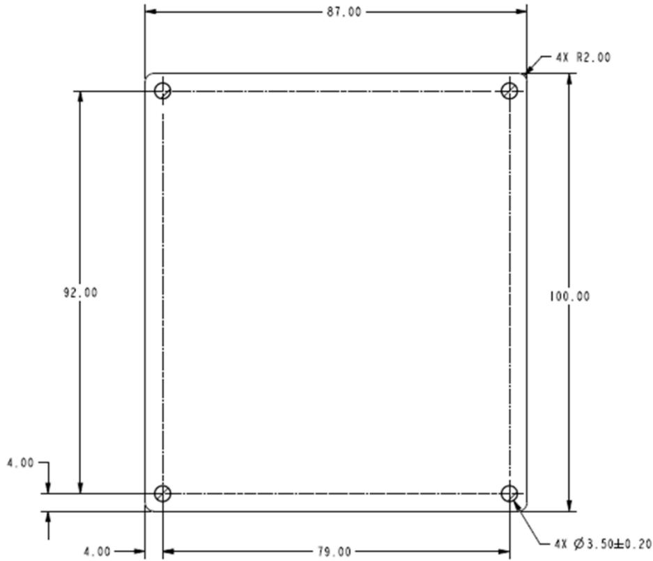
Figure 7-3. Module Mechanical Drawing - Side View
